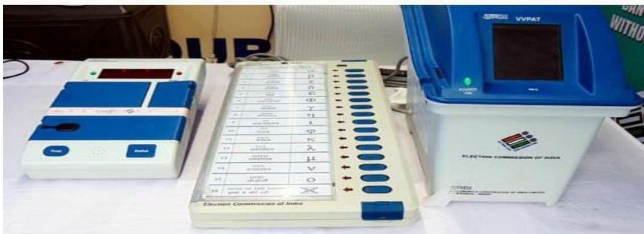
Fig 1.4: Electronic Voting Machine (EVM) with Voter Verifiable Paper Audit Trail (VVPAT)
